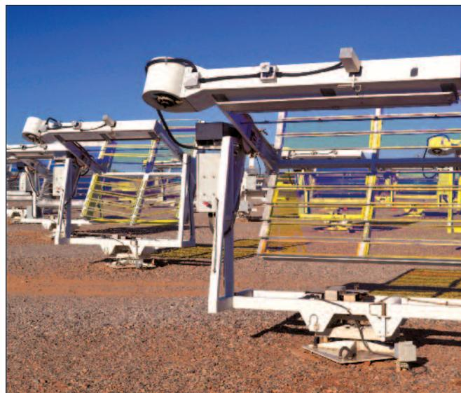
**The Atlas Low-Temperature EMMA uses a cool-mirror technology to accelerate exposure while keeping temperatures low (photo courtesy of Atlas Material Testing Technology).**
